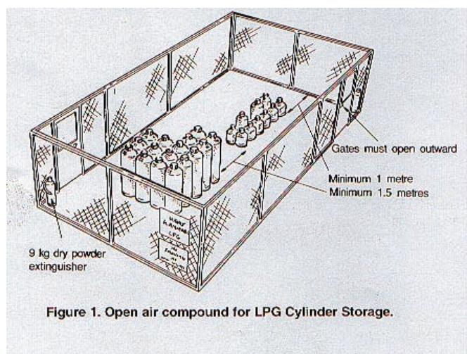
Figure 1. Open air compound for LPG Cylinder Storage.
